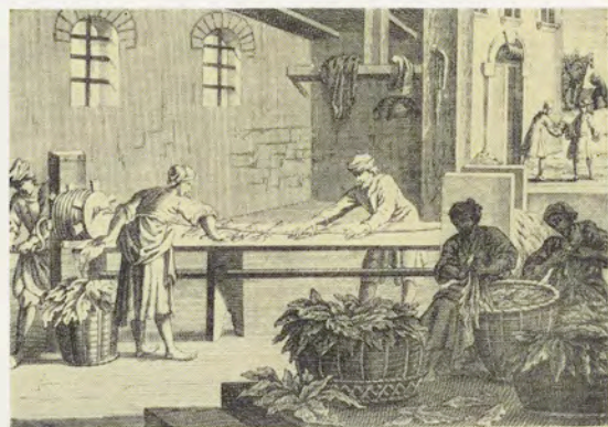
Tobacco leaves are being twisted into long, thin rolls in this early 18th century European factory
